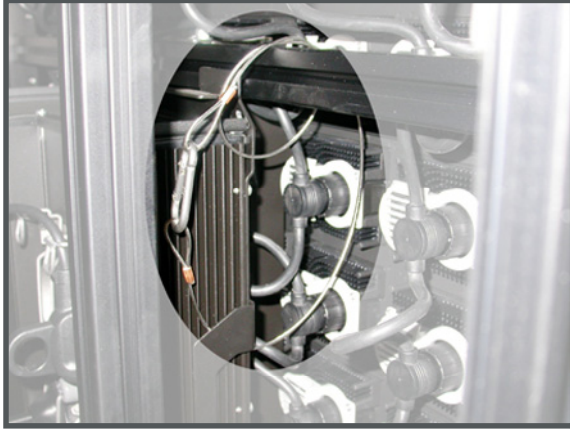
Image 12-4 Safety cable around the carrying handle and twice around horizontal profile.
